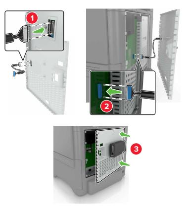
7 Reattach the controller board access cover.
