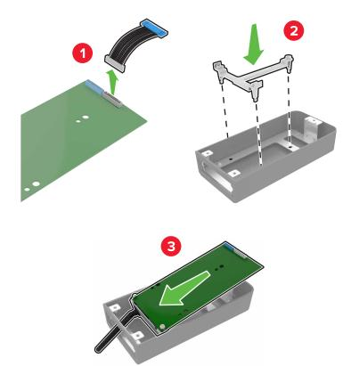
**5** Attach the housing to the controller board access cover.
